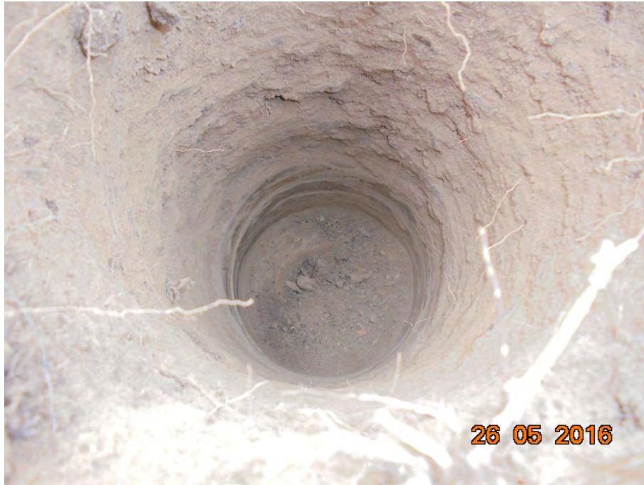
Photo 5 – Gravelly silty clay and sandstone in Bore 107
