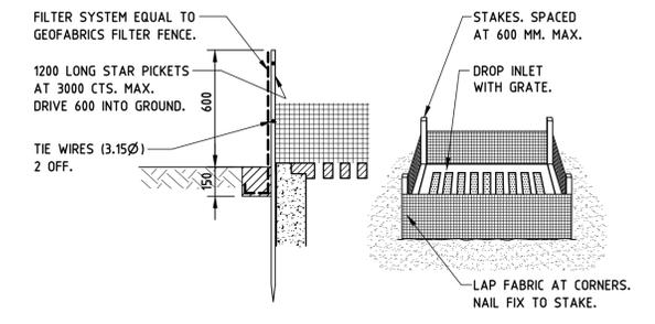
**GEOTEXTILE FILTER FABRIC DROP INLET SEDIMENT TRAP.**
