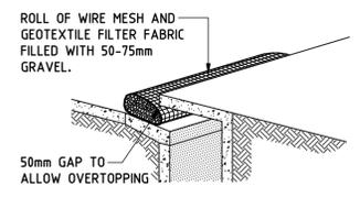
**PORTABLE GRAVEL KERB INLET SEDIMENT TRAP**
